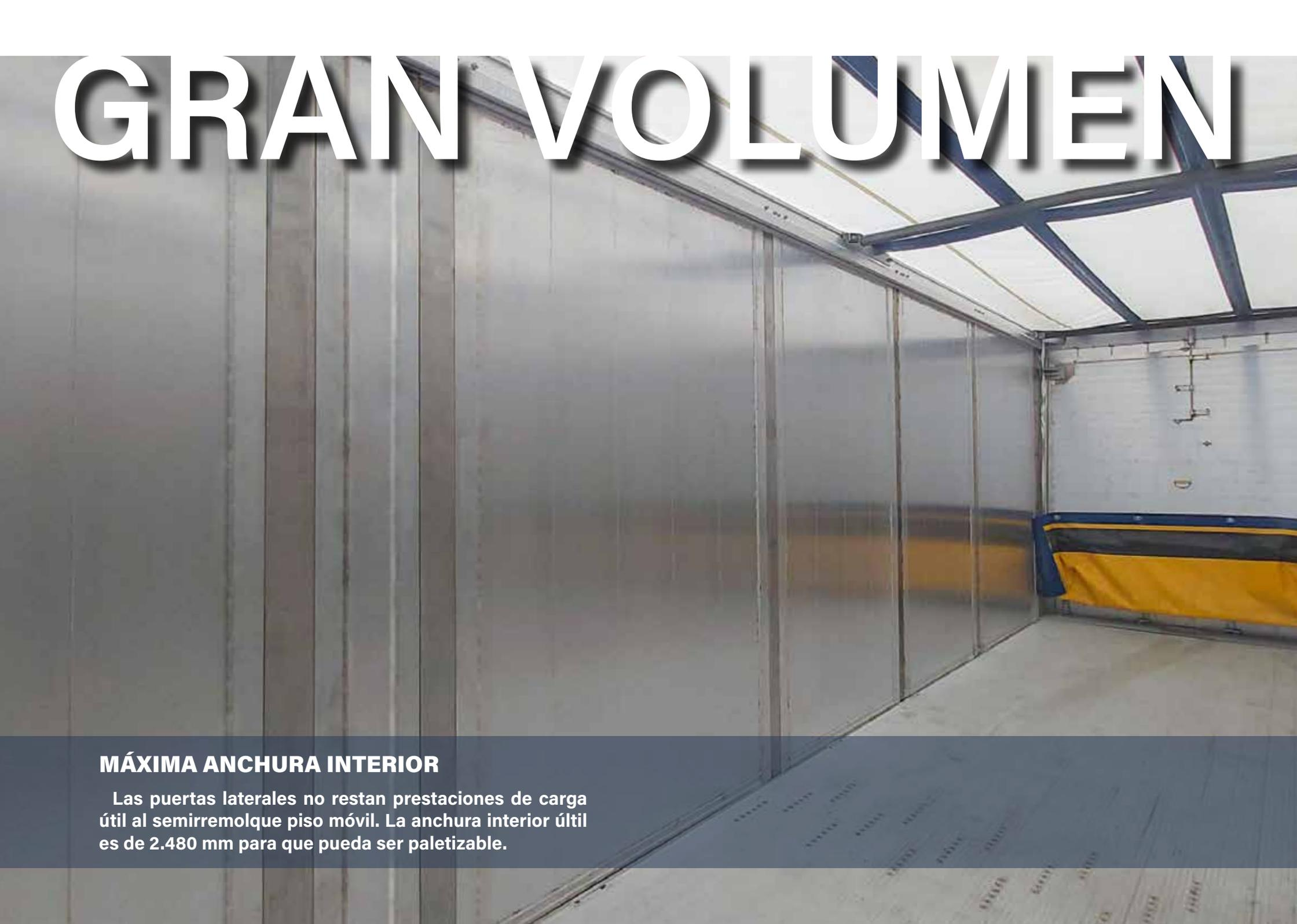
The image shows the interior of a semi-trailer. The walls are made of metal panels with vertical ridges. On the right side, there are several large sliding doors. The floor is a flat, light-colored surface. In the background, a blue and yellow tarp is visible, partially covering the rear of the trailer. The ceiling has a metal frame structure.
