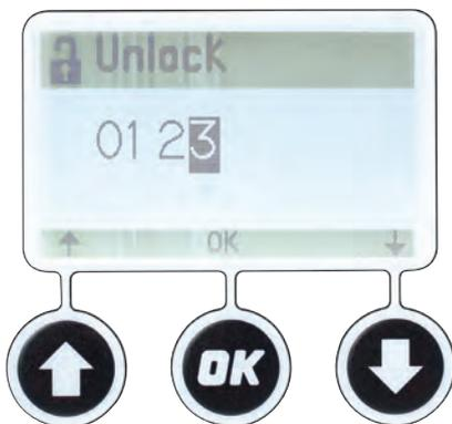
A PIN is used to protect a number of the EB+ Info Centre menus, as standard the EB+ Info Centre will be supplied with the PIN set to 0123.
