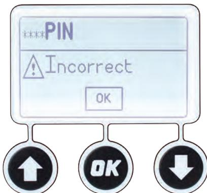
If any of the numbers entered into the unlock screen are wrong, the PIN Incorrect screen will be displayed.
