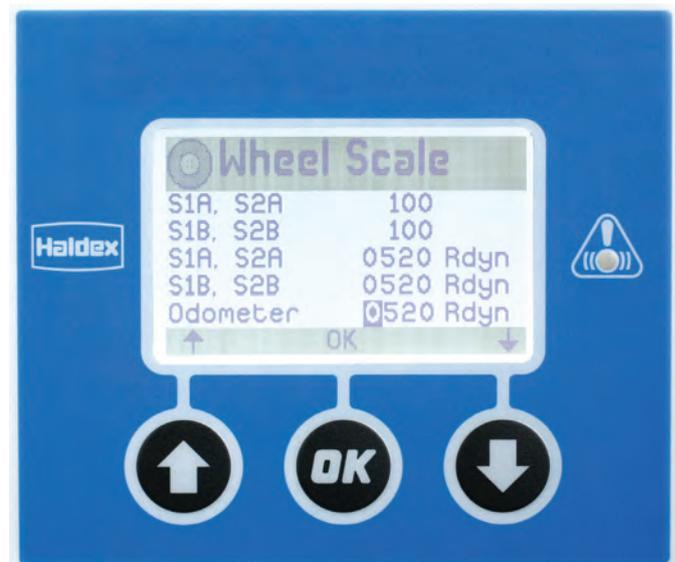
Use the button to exit the wheel scale menu without saving the data.
