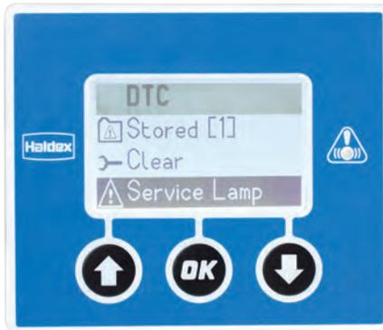
Displays the reason for the flashing trailer warning lamp.
