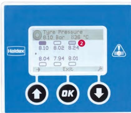
Use the button to move and highlight the faulty tyre.
