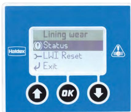
Displays the trailer brake lining wear condition.
