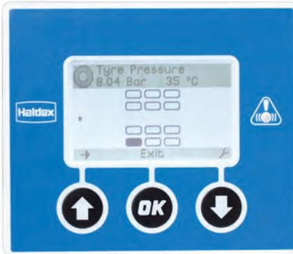
Use the button to display the highlighted tyre data.
