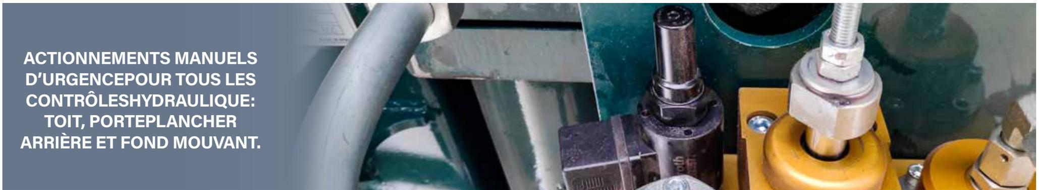
**ACTIONNEMENTS MANUELS D'URGENCE POUR TOUS LES CONTRÔLES HYDRAULIQUES: TOIT, PORTEPLANCHER ARRIÈRE ET FOND MOUVANT.**
