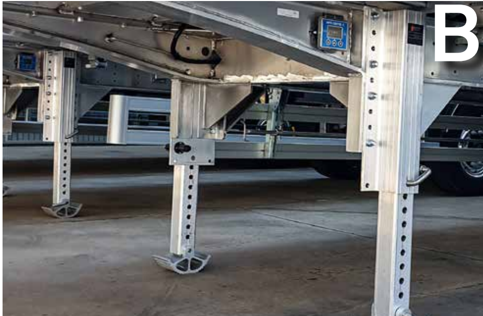
ALUMINUM LEGS WITH MANUAL EXTENSION
