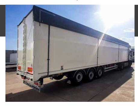
The models of the Conical Half family mount the 385/65 R22.5 wheel and offer you the highest possible load volume thanks to its lowered chassis and the maximum conciseness of its body.
