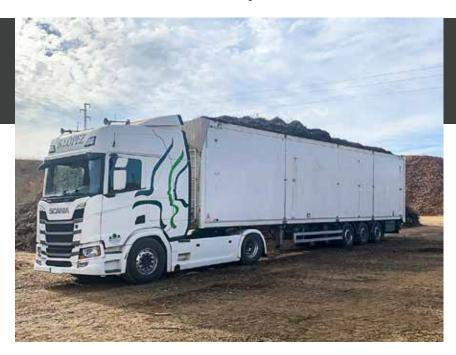
The models of the Conical Full family mount the 385/55 R22.5 wheel and offer you the highest possible load volume thanks to their lowered chassis and the maximum conciseness of their bodywork.
