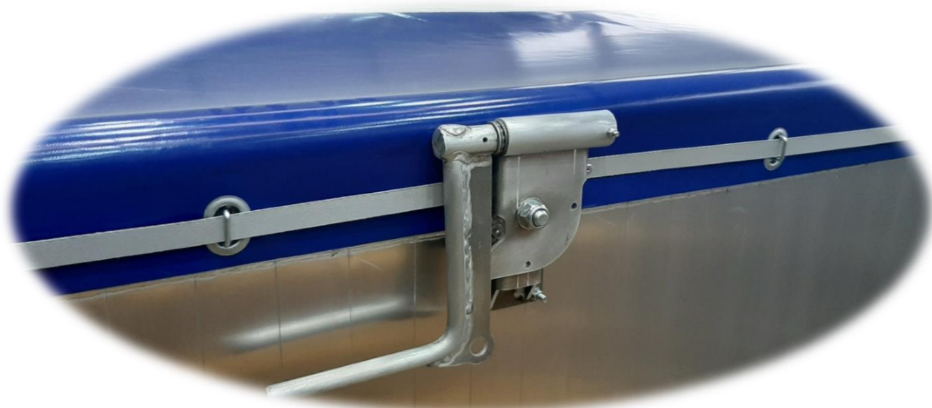
DETAIL OF THE LOWERED BAYONET IN RUNNING ORDER WITH LOCKING BY MECANIC BALL POSITIONER.
